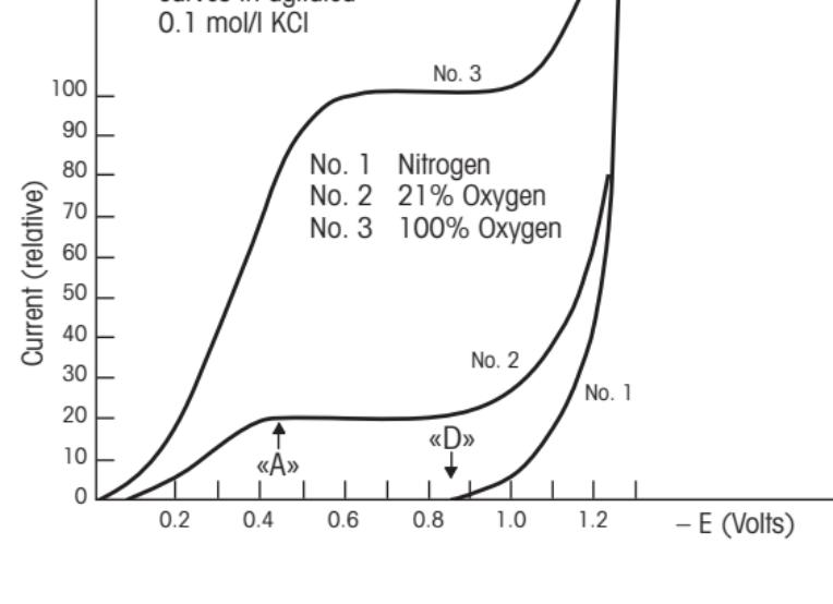
The polarization voltage should remain as constant as possible. Besides a constant source of voltage the following prerequisites must be met: The electrical resistance of electrolyte film must not exceed a particular value so as to avoid a voltage drop.
