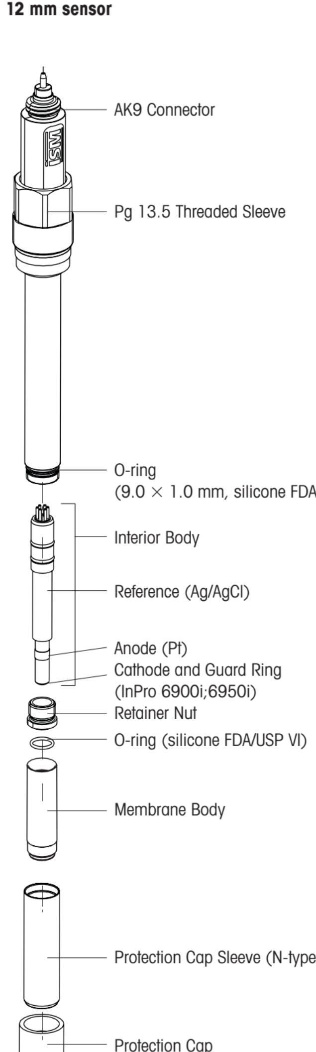
METTLER TOLEDO ISM O<sub>2</sub> sensors are supplied with fitted membrane body but without electrolyte and covered with the protection cap and have been checked for proper function.
