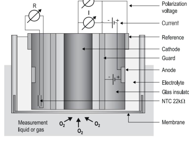
As a consequence of the reaction at the cathode and the anode, a current flows between cathode and anode (4 electrons per oxygen molecule), which is proportional to the oxygen partial pressure at the cathode.
